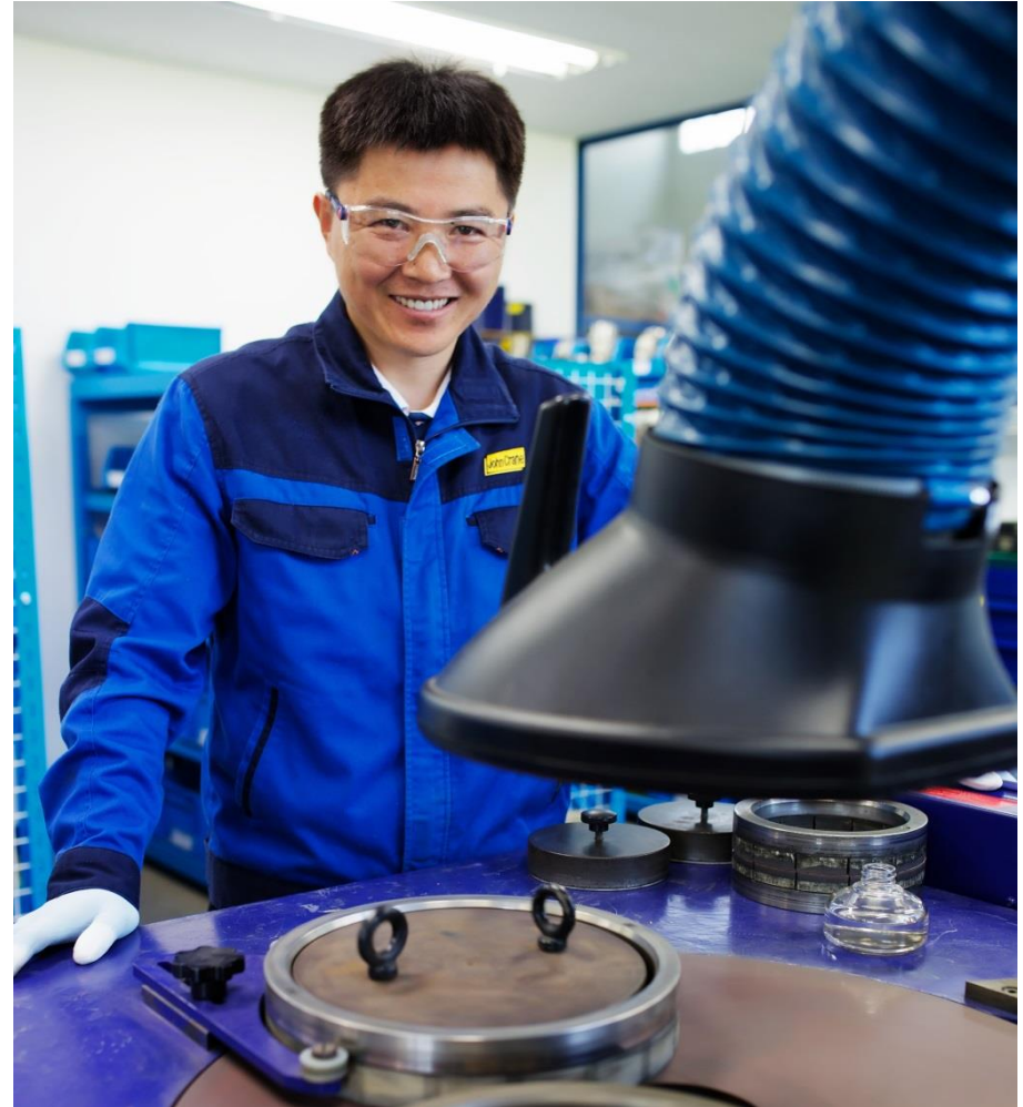
> Precision lapping mechanical seal face in Busan, South Korea service centre
