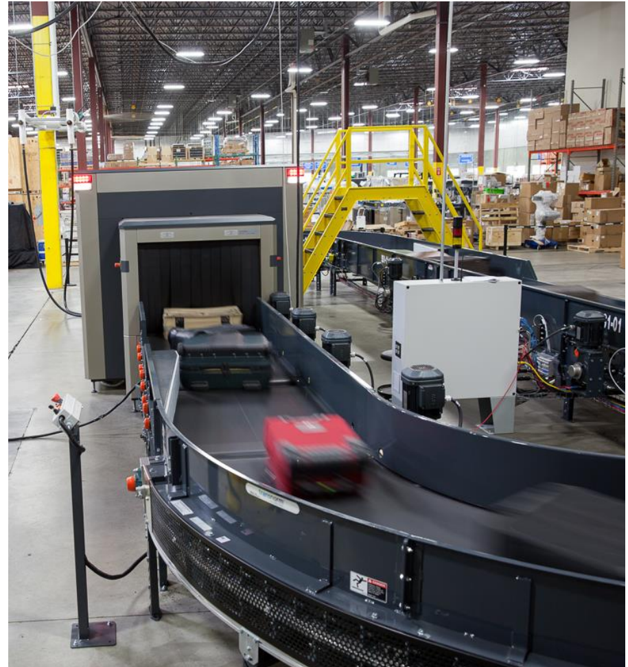
> Next generation high-speed checked baggage scanner, can screen up to 1800 bags an hour
