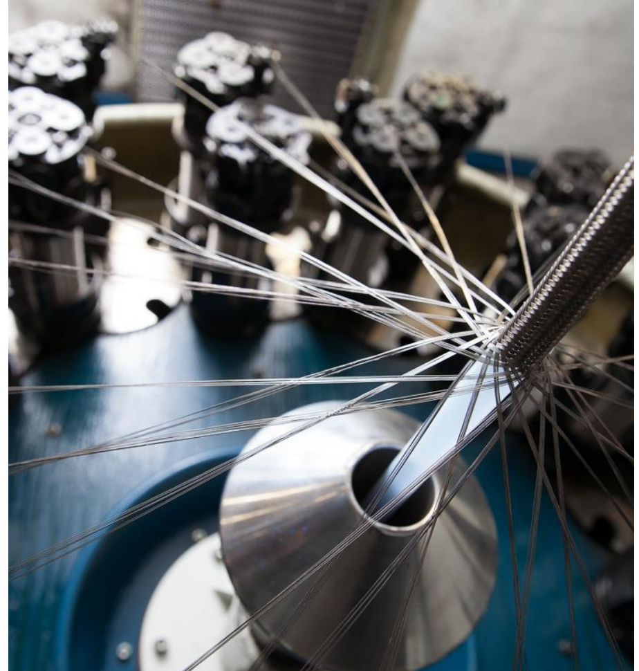
> Precision stainless steel braiding provides protection and strength for high pressure Teflon® tubing
